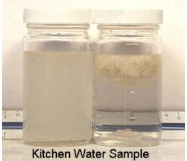
The Oil/Water sample was received at a pH of 8.5. The sample was treated with Floc at a dosage of 0.1 gram/100ml or 8.3 lbs/1,000 gallons. Note the drop in TDS/Conductivity.
