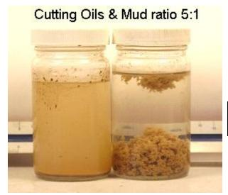
The 1 part Drilling Mud to 5 parts Cutting Oils wastewater sample was at a pH of 6.5. The sample was treated with Floc™ at a dosage of 0.1 gram/100ml or 8.3 lbs/1,000 gallons.
