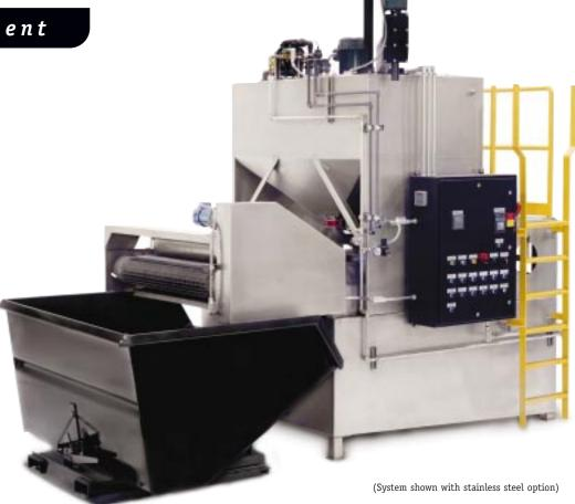
Ringwood's wastewater treatment units optimize the use of clay based flocculants to clarify industrial wastewaters.
