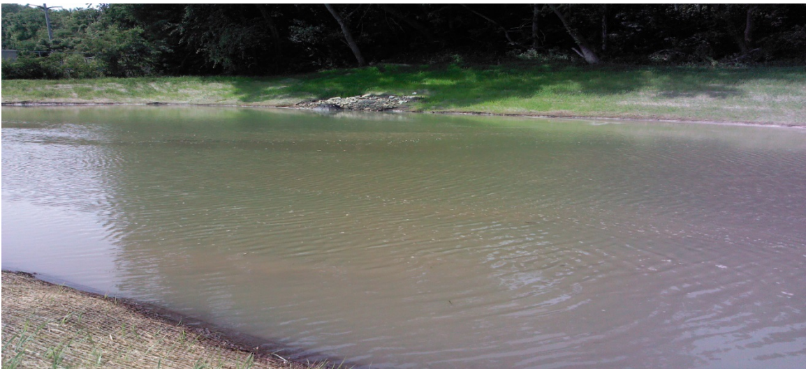
5 minutes after FLOC treatment-FLOC applied at 11:00 a.m., 1:00 p.m. 12.5 NTU
